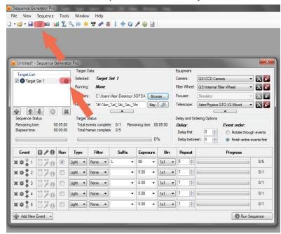
table, make sure there is a check mark on the "Run" box. Under Filter, tell it you want your Lum filter, Give it the Suffix Lum, and give it an exposure of 60 seconds. Bin 1 x 1 (or ISO 400 on DSLR) and tell it to repeat five times. Make sure no other event boxes are checked. (If using a one shot camera like a DSLR, don't name a filter.)
